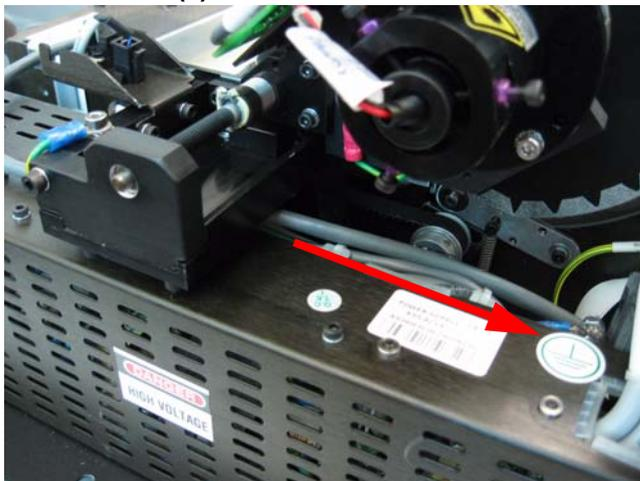
Pass the cable around to the Motion card (3)
