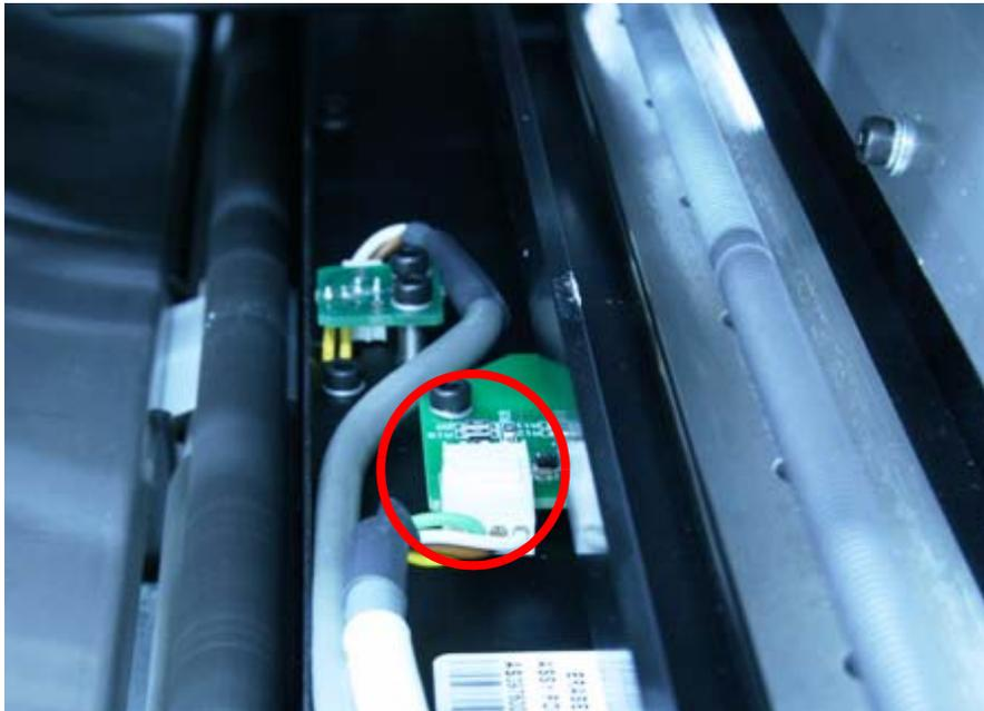
[3] Disconnect the cable from the Erase Lamp Sensor.
