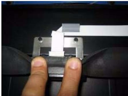
[6] Release the two Allen screws holding the Key Assembly from the left and the two Allen screws holding the Key assembly from the right and cut the protective sponge strip.
