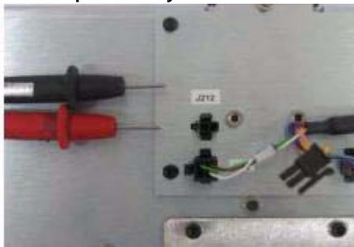
If the resistance values are incorrect, replace the solenoid.
