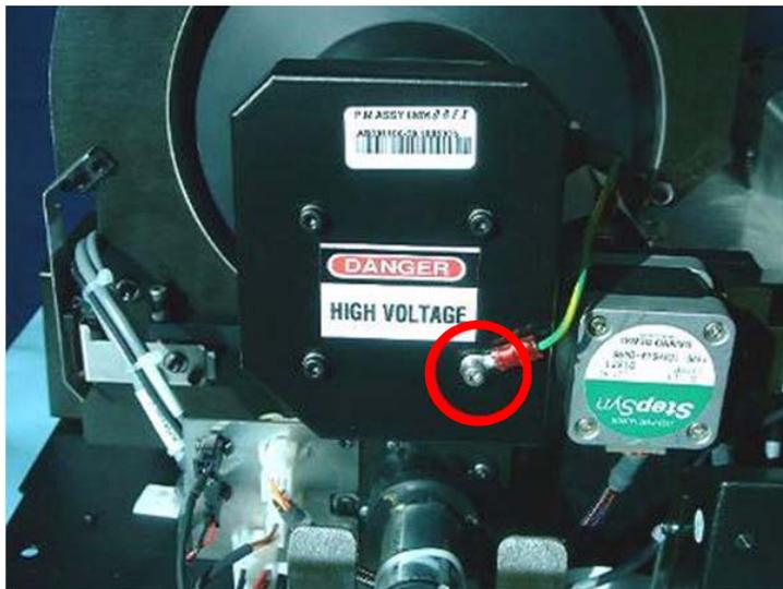
[3] Disconnect the 3.0 mm Ground wire connector to the Slide body from the PM Tube.
