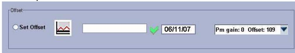
[4] The offset calibration ends. A green check mark should appear next to the offset calibration field.
