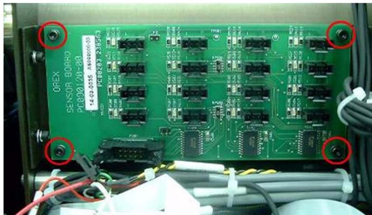
[3] Remove the four 2.5 mm Allen screws securing the Sensor Board.
