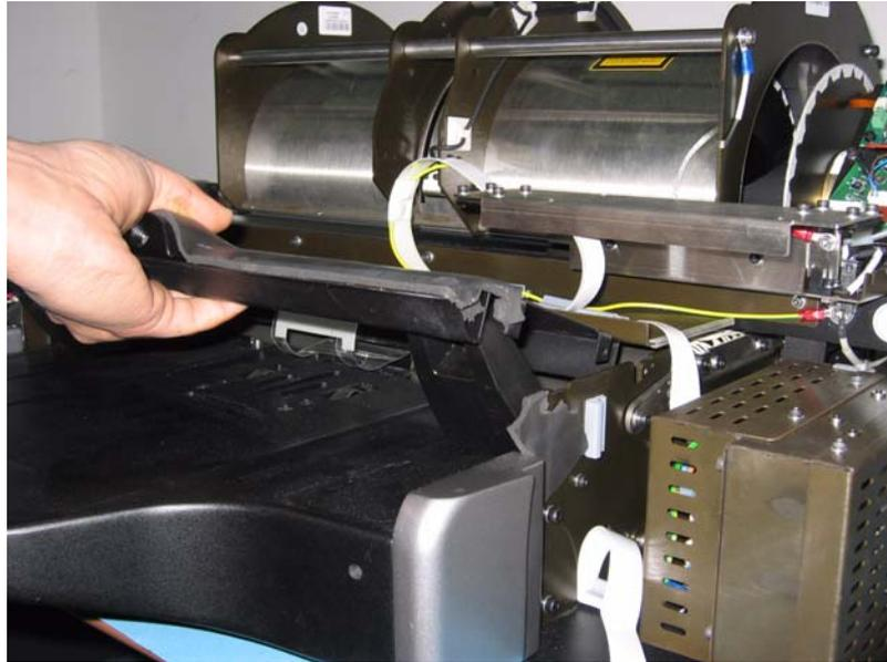
[8] Remove the two Allen screws attaching the Screen Guide bracket to the Key Assembly, releasing the old Screen Guide.
