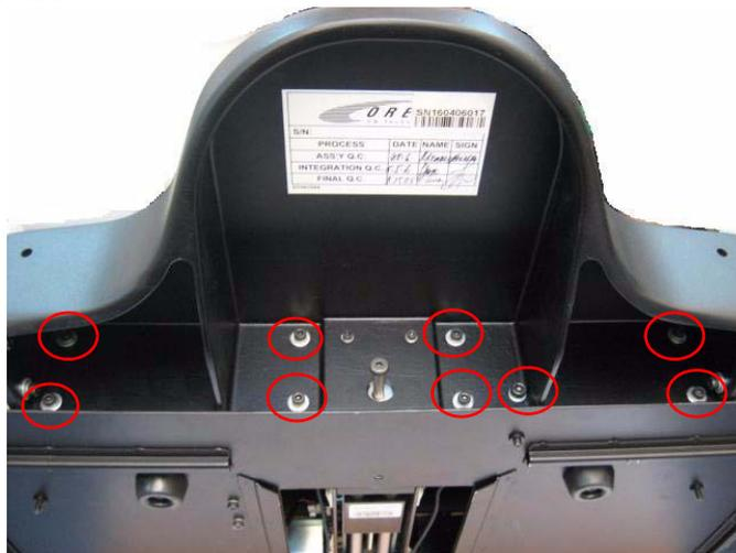
**[8]** Remove four M3 screws holding the plate sides (two on the left side and two on the right) and remove them.
