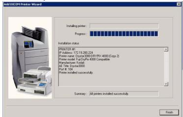
*Kodak* Point-of-Care CR System is ready for DICOM print after a DICOM printer is successfully added. The printer information appears in **Start>Setting>Printers and Faxes**.
