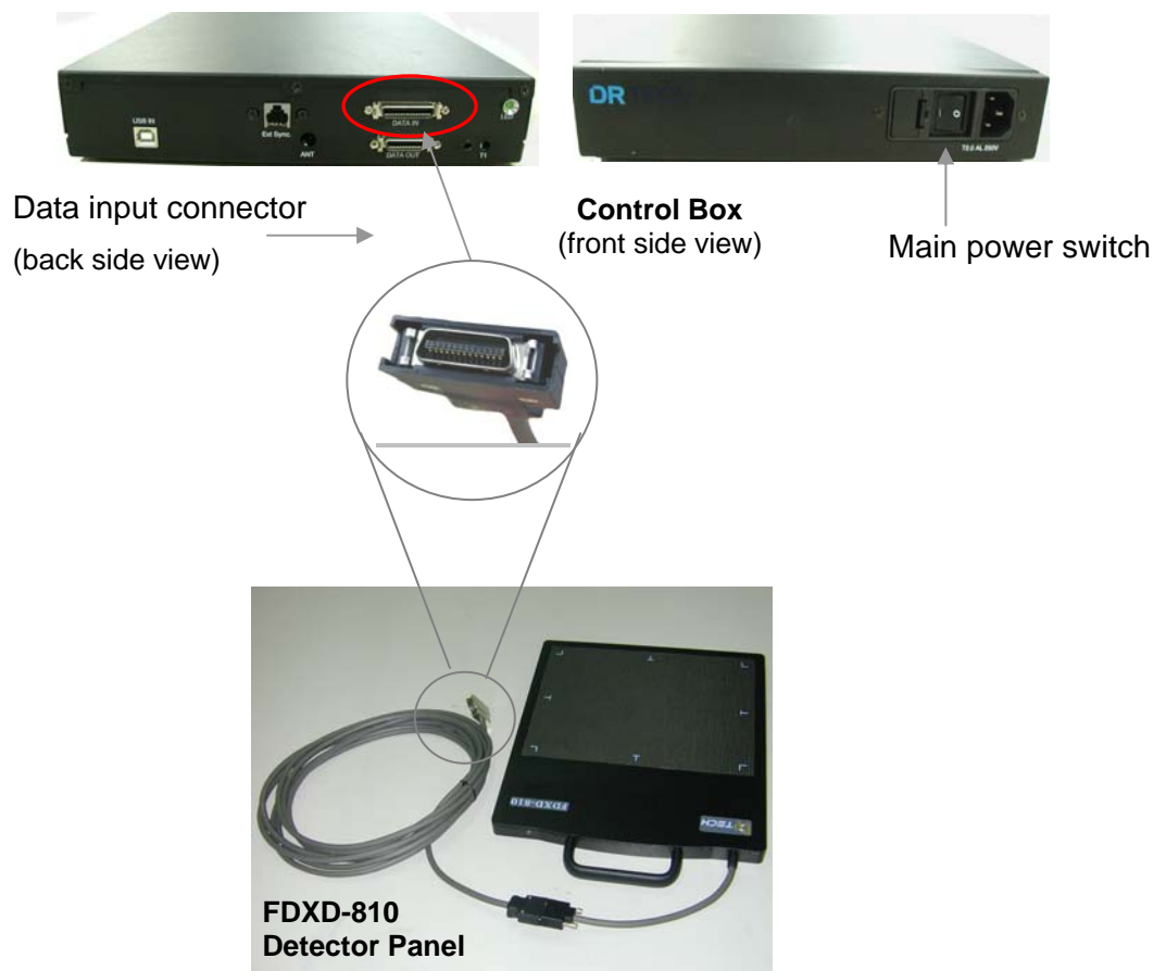
Figure 4-1. Detector Panel and Control Box interconnection
